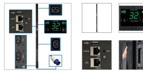
7.7kW 0U PDU distributes and monitors single-phase power in an IT or industrial environment. Built-in Java-free network interface helps you remotely monitor load levels to prevent overloads that cause downtime.
